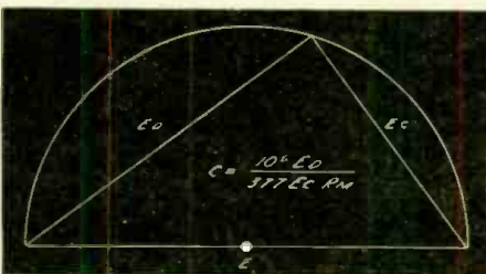
Fig. 9—Meters may be calibrated without recourse to cut-and-try, using the chart above.
