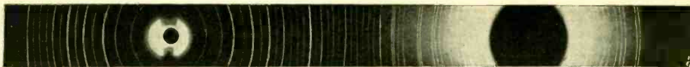
Above, the diffraction pattern for tungsten; on opposite page, that for copper. Line spacing and brightness identifies the material.
